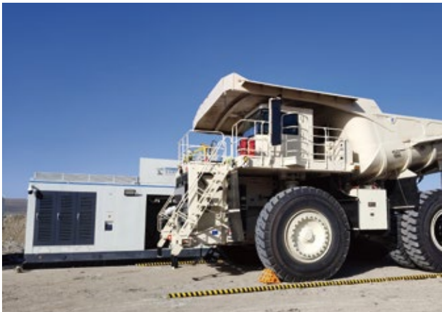
World's First 4.5MW Dual-Gun Automatic Charging System
